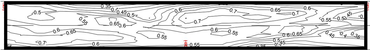
**Fig. 9** – Luminance calculation (Philips Calculux Road 5.0)
