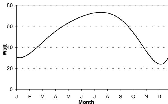
**Fig. 10** – Power potential of the system (PV panel fixed at 55°)
