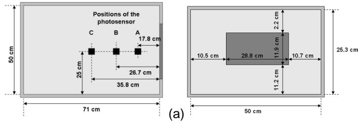
Figure 3. Floor plan of the scaled room with the various measurement positions (a) and south façade of the scaled room (b).
