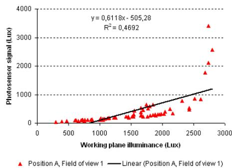
Figure 7. Ceiling illuminance (photosensor signal) at position A with FOV 1 vs. working plane illuminance (total number of days with clear and diffuse glazing April - May 2007).
