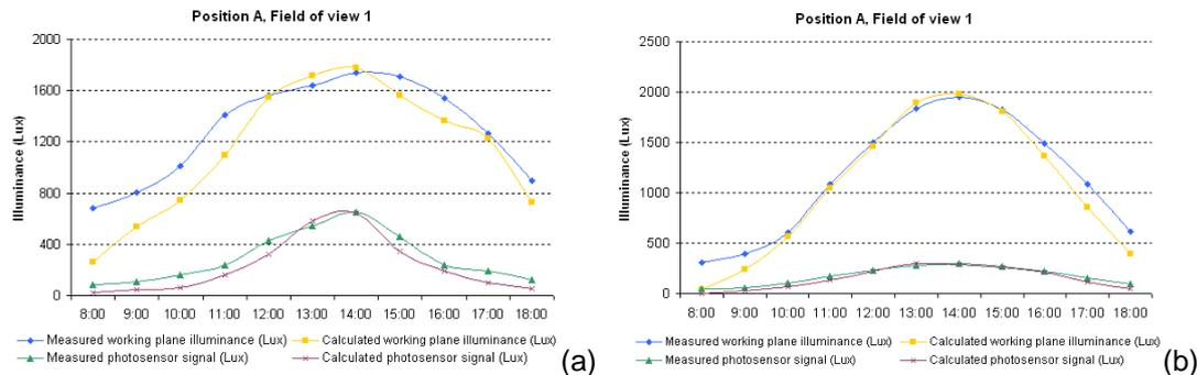
Figure 9. Distribution of measured and calculated illuminance values within 8:00 to 18:00 LT, between working plane and ceiling for position A and FOV 1 (15/05/2007) (a) and with diffuse glazing (27/04/2007) (b).
