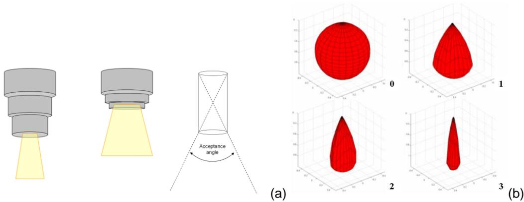
Figure 1. Variable FOV of sensor using a telescopic cylinder (a) and spatial responses for the selected adjustments of the telescopic cylinder (0 corresponds to a spatial response without the telescopic cylinder) (b).
