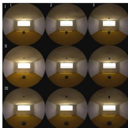
Figure 8. Radiance hemispherical images from scaled model interior. The three rows correspond to the respective sensor positions (A, B, C) and the three columns to the respective sensor cover geometries (FOV 1 to 3).
