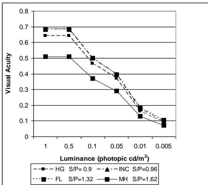
Figure 4. The visual acuity versus luminance for the various lamps and ratios S/P.
