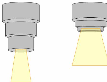
Figure 2. Photosensor with telescopic cylinder that can be altered from a sensor with narrow view in a sensor with wide field of view
