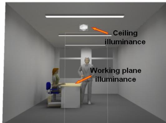
Figure 1. Working plane and ceiling illuminance inside a room with photosensor
