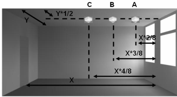
Figure 6. View of the room with the positions of the photosensor from the window
