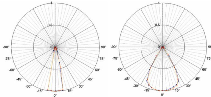
Figure 3. Polar diagrams of spatial response of the new developed photosensor with narrow and wide field of view with the help of the telescopic cylinder
