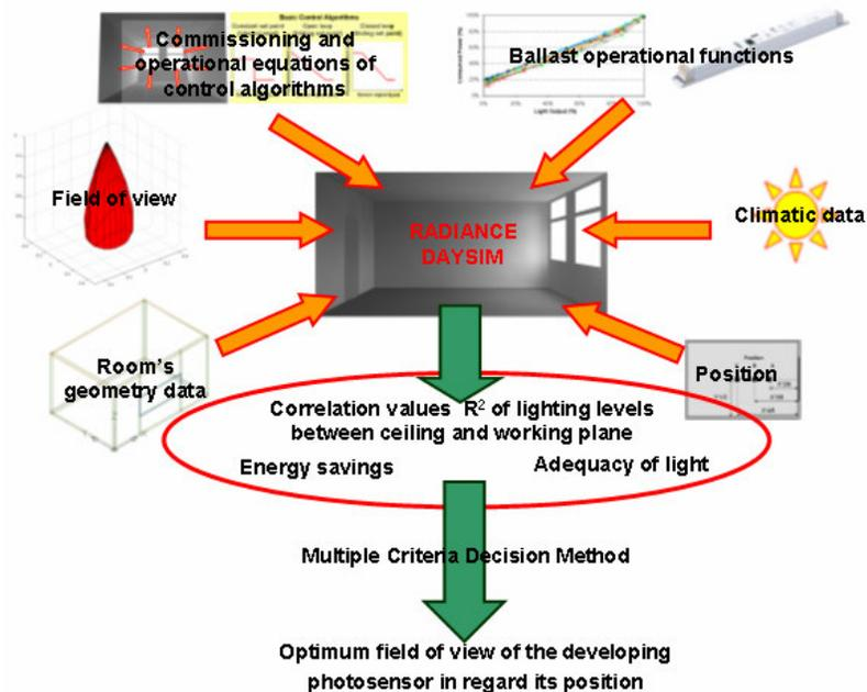
Figure 5. Diagram of the methodology for the optimisation of the placement of the photosensor
