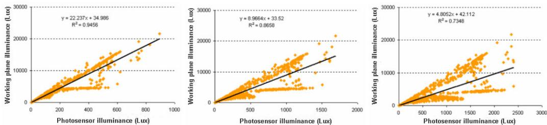
Figure 4. Lighting levels and the corresponding  $R^2$  values between the working plane and the ceiling for the photosensor with narrow, medium and wide field of view (from left to right)
